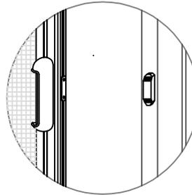
ATTACH THE MAGNET PLATE TO THE LEADING EDGE OF THE SCREENS PULL BAR, AND THE MAGNET ON TO THE SIDE OF THE DOOR FRAME, OR MOLDING.
